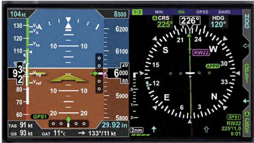
Figure 4.6 - Same EFIS display with a 50% reduction in colour
