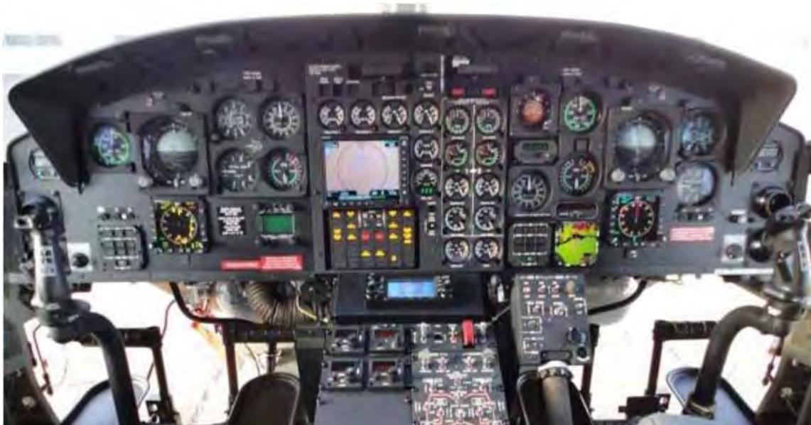
Figure 4.7 - BELL 412 Standard Instrument Panel – Full Colour
