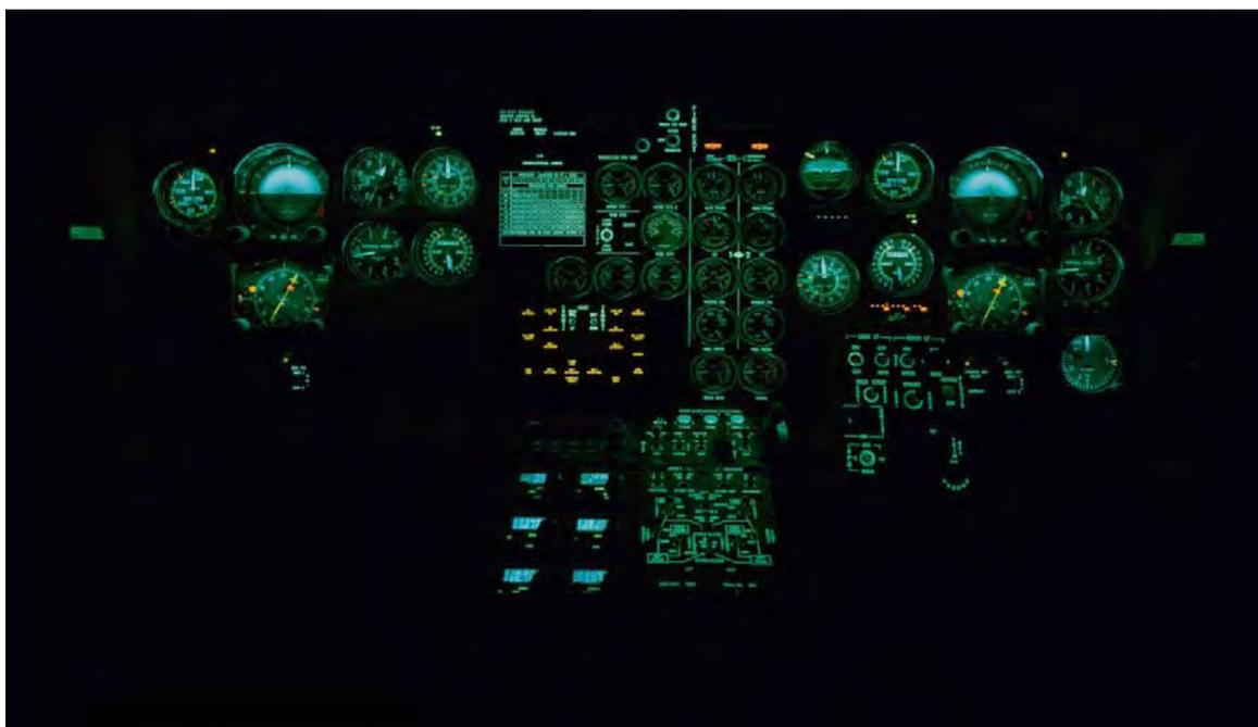
Figure 4.8 - BELL 412 Standard Instrument Panel – Equipped for Night Vision Goggles (NVG). All flight, engine and performance instruments are monochromatic (Green)
