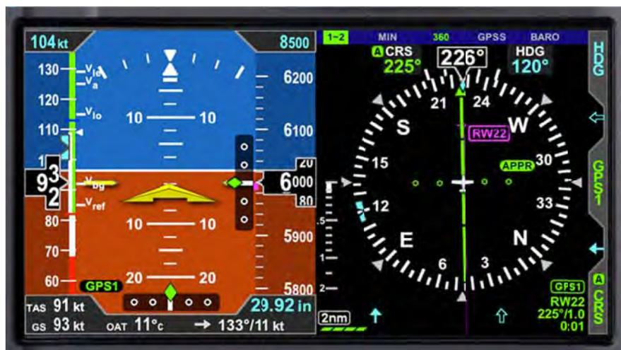
Figure 4.5 - EFIS display of attitude indicator and horizontal situation indicator
